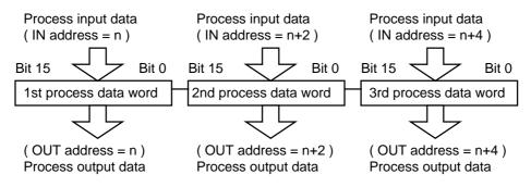
Figure 11: Arrangement of the data registers of an InterBus-S device
