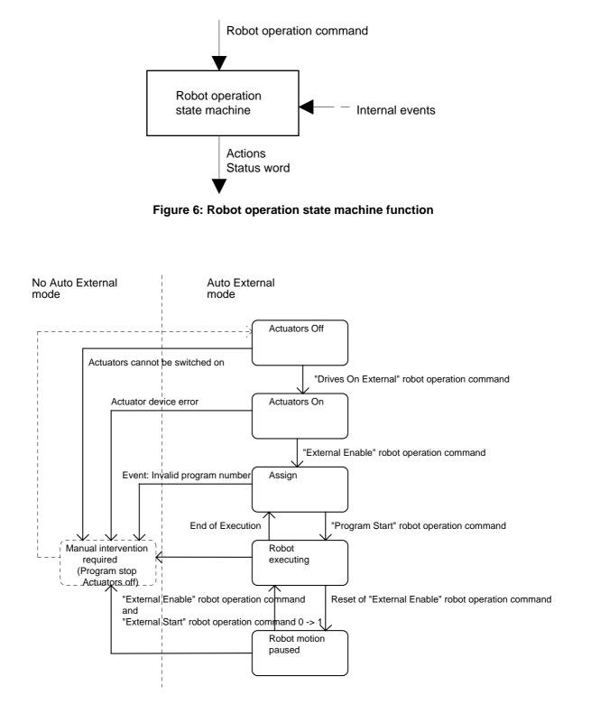
Figure 7: Robot operation state machine
